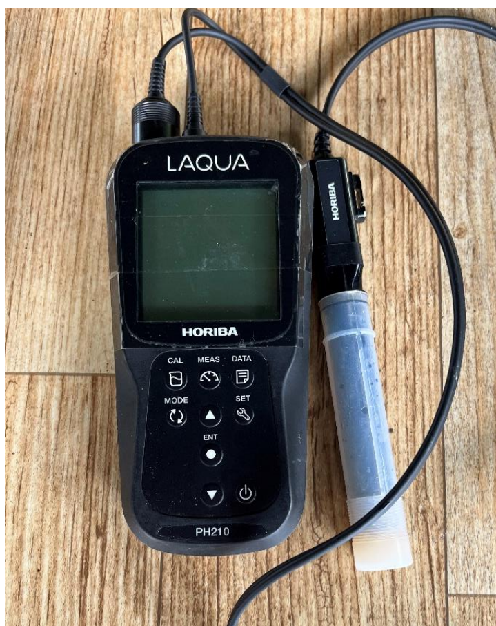
Figure 7. Horiba LAQUA pH210 pH/ temperature meter was used for measuring pH and temperature directly at site.
