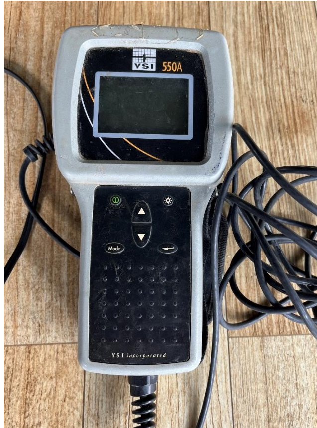
Figure 8. YSI 550A dissolved oxygen instrument was used for measuring dissolved oxygen directly at site.
