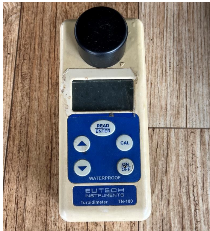
Figure 9. Eutech Tn100 turbidity meter was used for measuring turbidity at site.
