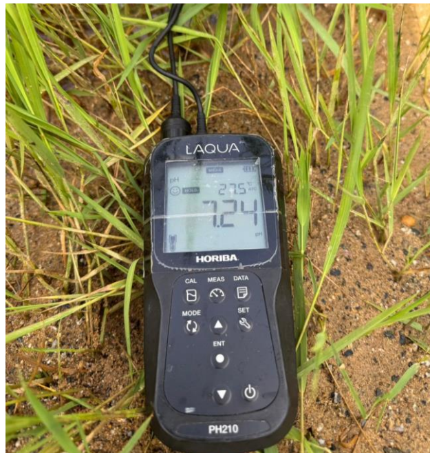
Figure 9. Horiba LAQUA pH210 pH/ temperature meter was used for measuring pH and temperature directly at site.
