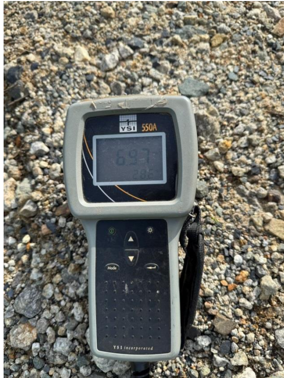
Figure 10. YSI 550A dissolved oxygen instrument was used for measuring dissolved oxygen directly at site.
