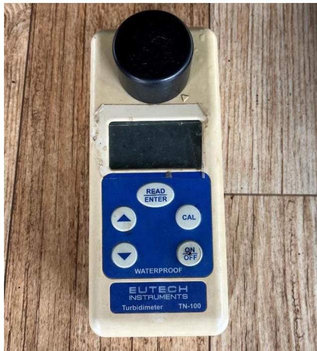
Figure 11. Eutech Tn100 turbidity meter was used for measuring turbidity at site.
