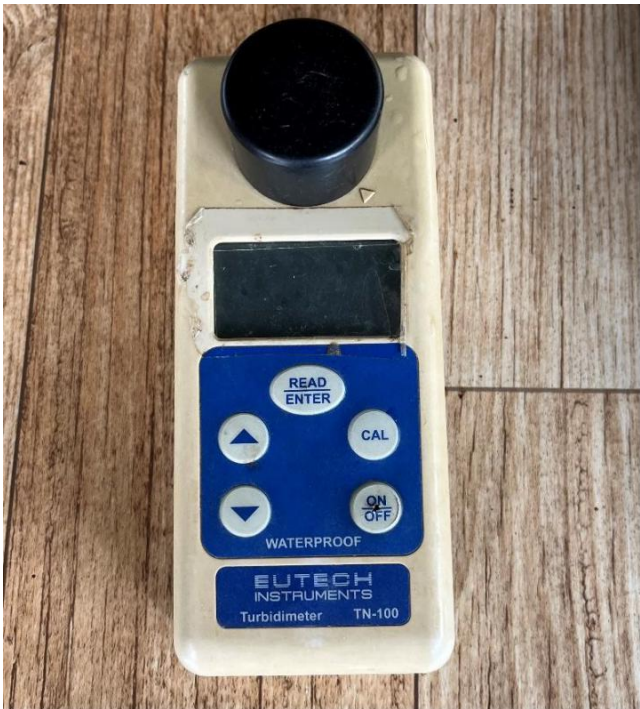
Figure 12. Eutech Tn100 turbidity meter was used for measuring turbidity at site.
