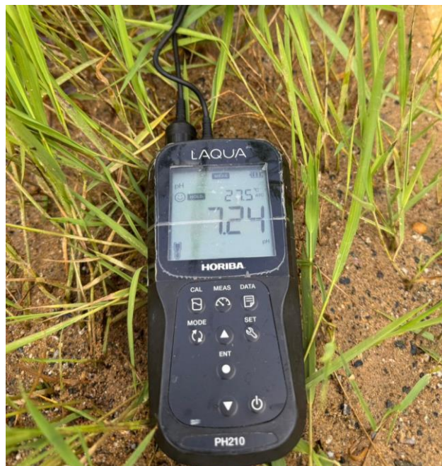
Figure 10. Horiba LAQUA pH210 pH/ temperature meter was used for measuring pH and temperature directly at site.
